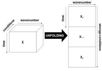
Fig. 1. Unfolding procedure of the X three-dimensional matrix of spectra.
