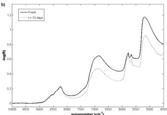
Fig. 3. Spectra of body lotion products stored for different times and at distinct conditions. (a) No baseline correction applied; (b) baseline offset removed for clarity.
