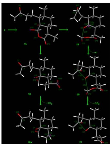
Figure 10. Reaction routes B2 (left) and B3 (right). Interatomic distances involving O1 and bond angles around radicals at C9 and C12a are shown for 18a and 19-21. Pink balls, ball halves and dashed lines show radical localization or partial delocalization.
